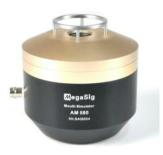
Artificial Mouth 580 is designed for accurate and repeatable electroacoustic measurements. It has extraordinary distortion performance, typical value is: after equalization to 94dBSPL, 25mm distance, the THD can be lower than 1%.
